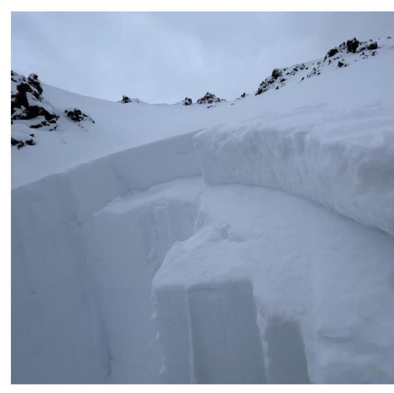
While investigating an avalanche that failed on a weak layer of facets buried in January, we notice a new layer that we will be looking for and testing as we move forward. Photo: GNFAC
